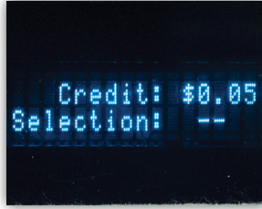
Vacuum Fluorescent Display With point of sale message and credit display options.
