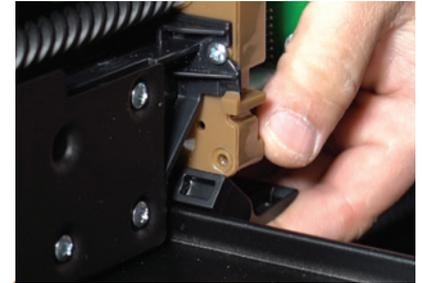
Each module is self contained and has unlimited adjustments using a pinch lever on the back of the unit. Re-configure a selection in seconds.
